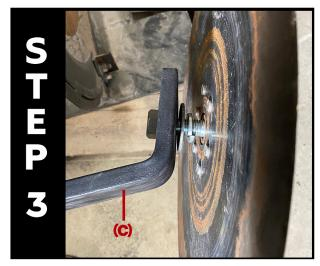
After placing 5/8"x2-1/2" bolt into disc blade, place lockwasher then flat washer (as shown) onto bolt before placing bolt into bracket (C). Tighten locknut.
