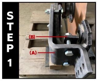
Fasten large bracket (A) to 28% arm using (4) 1/2"x2-1/2" bolts. Place offset bracket (B) as shown.
