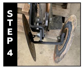
Place both disc blades onto Bracket (C). (Recommend starting in bottom hole)
