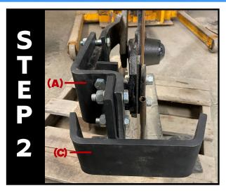
Bolt disc bracket (C) to large bracket (A) using (2) 1/2"x2" bolts.
